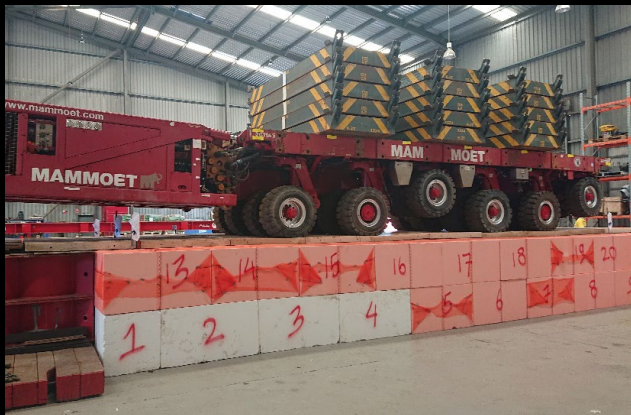
SPMT and temporary fill trial in Netherlands
