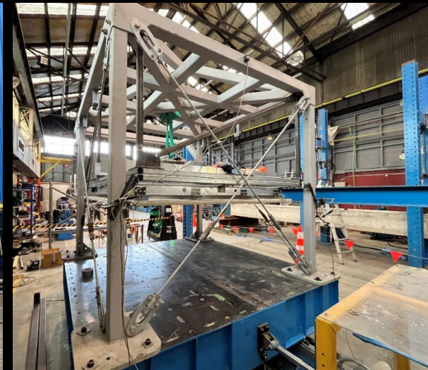
Ceiling shake-table test in NZ
